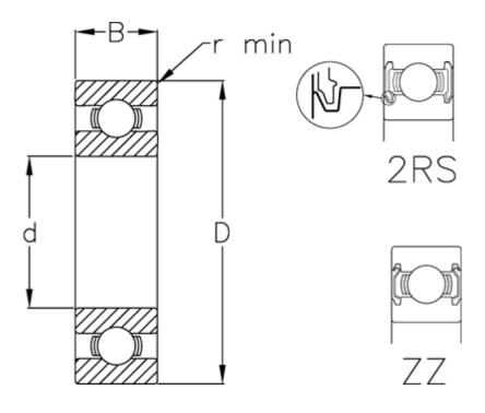
B = 12 d = 50 D = 72 Dynamic load C (kN) = 15.6 Max rpm greased = 8900 Max rpm oil lubricated = 11000 r min = 0.6 Static load C0 (kN) = 12.2
